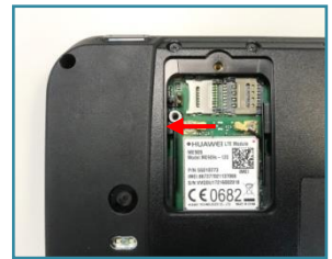
Figure 4 Close the lid and follow the direction to lock.
