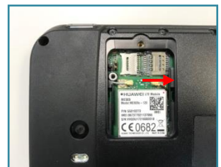
Figure 7 Close the lid and follow the direction to lock.
