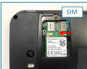
Figure 5 Follow the direction of red arrow to open the lid of SIM slot.
