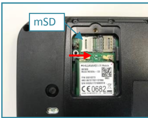
Figure 2 Follow the direction of red arrow to open the lid of mSD slot.
