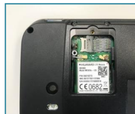
Figure 6 Open the lid and insert the SIM card into the slot.
