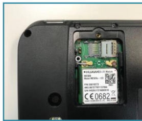
Figure 3 Open the lid and insert the mSD card into the slot.
